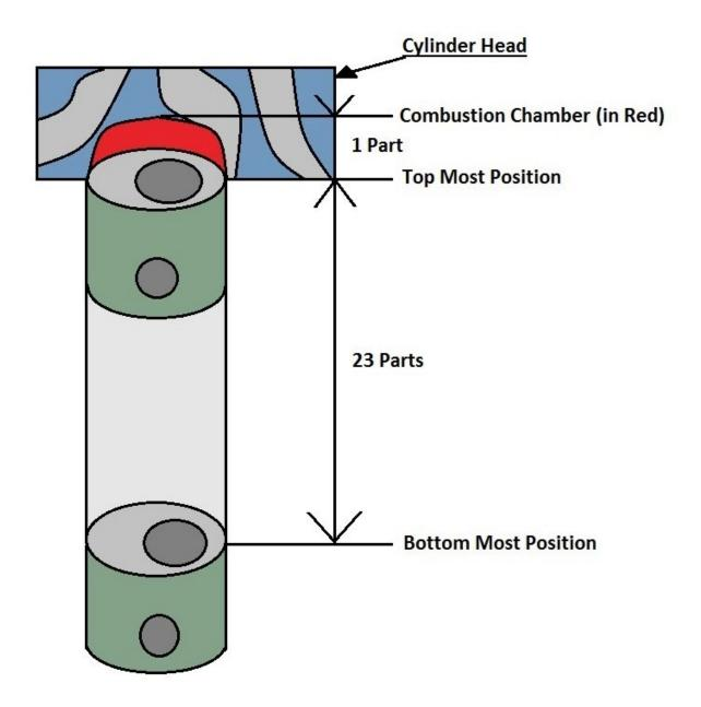
Compression Ratio = 23:1 (Diesel Engine)
