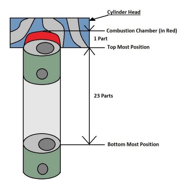
Compression Ratio = 23:1 (Diesel Engine)
